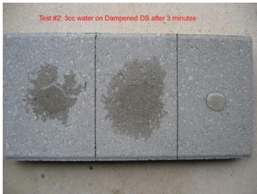
After 8 minutes, the center section has continued to grow as the water spreads out horizontally because the Deep Seal is blocking it from going down into the slab.
