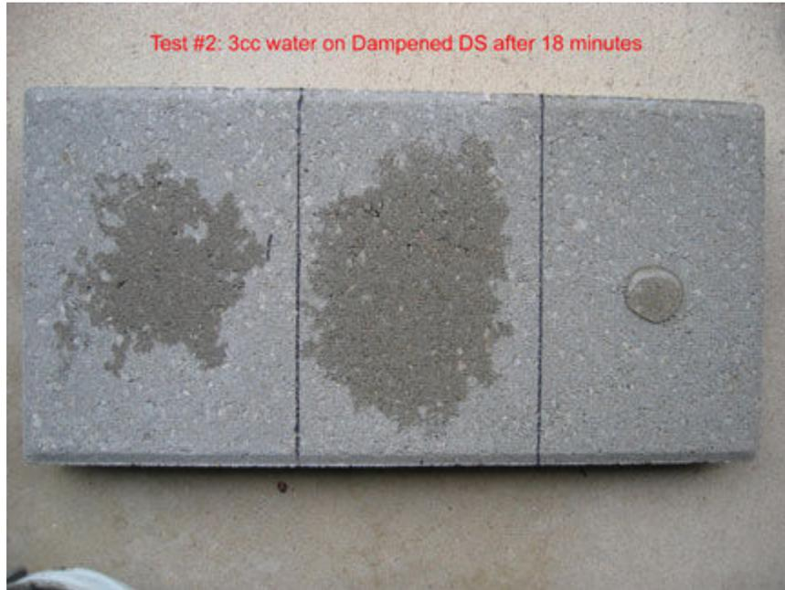
After 22 minutes you can notice that the middle section is starting to lighten up in color around the edges and at some places in the darkened (wet) area... the bare section on the left is not showing this lightening or drying.
