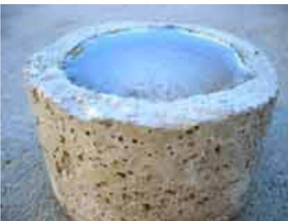
The container above was formed from just hand mixed cement, poured into a form, then a pop can pushed into it to make a cup like concrete container. It was treated with Deep Seal and Top Seal. As you can see the concrete is porous...however it holds the water and in fact, the water is arched into a bead inside the container. This will hold water... absolutely no absorption at all for extended periods.
