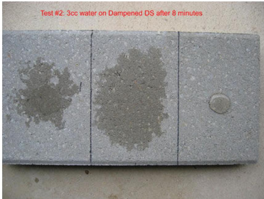
While hard to see at this resolution, there is still slight moisture on the surface in the two left sections, bare and DS only... the beaded 3 cc.s on right on the DS/TS has not changed at all.
