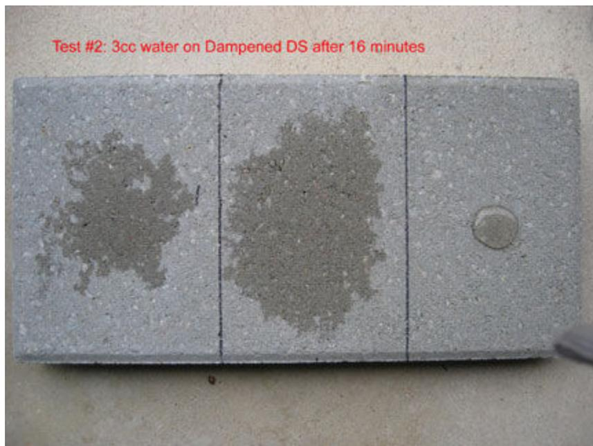
By 18 minutes, there is no water on the surface, it has all soaked in on the bare section and spread out wider in the middle section where the DS blocks the penetration under the surface. This illustrates that Deep Seal does NOT put a film on the surface, instead the top 1-2 mm are devoid of product and constitute a "bondable" surface for the application of adhesives, paints, surface coatings, overlays, stampwork etc.
